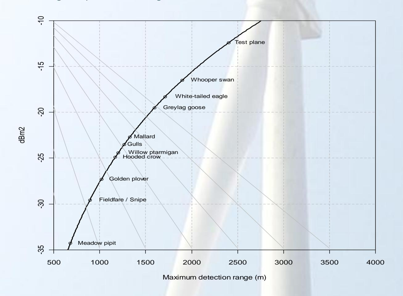
While the specific performance results obtained in these tests at Smøla are highly site and system/setting dependent, the method used should be universal and therefore possible to employ for other similar sites and types of radar equipment.
